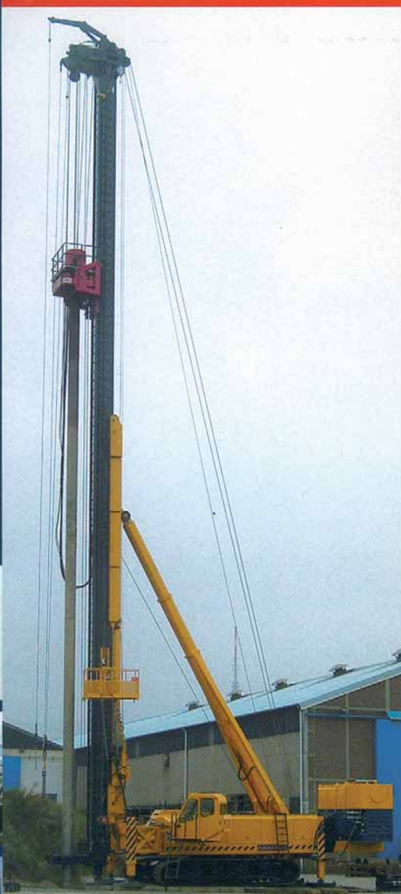
F3500, Hydraulic foundation machine
